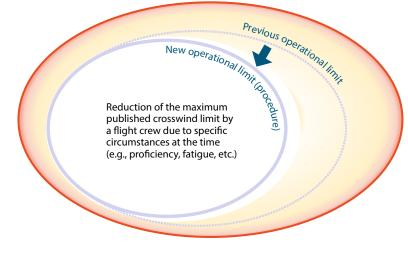
Figure 3: Remaining Within the Prevention Space Pattern of Operational Resilience by Modifying the Operational Limits
